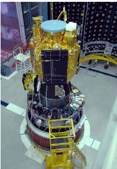
Figure 5 Polar Satellite Launch Vehicle Upper stage showing CubeSat deployers (picture courtesy of ISRO)
