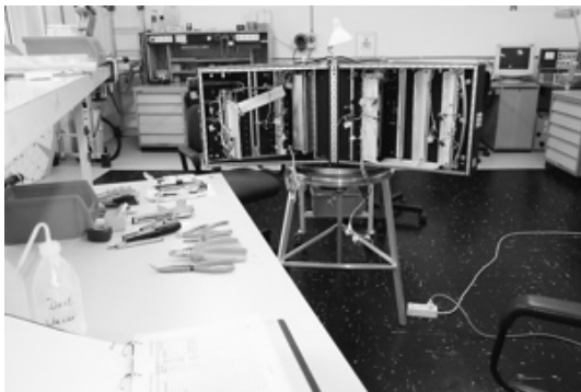
13. A current view of the satellite. The cables are drawn (?) connectors (?) are fitted and labelled. Everything is ready for the installation of the flight modules, some of which are ready and waiting in Marburg
